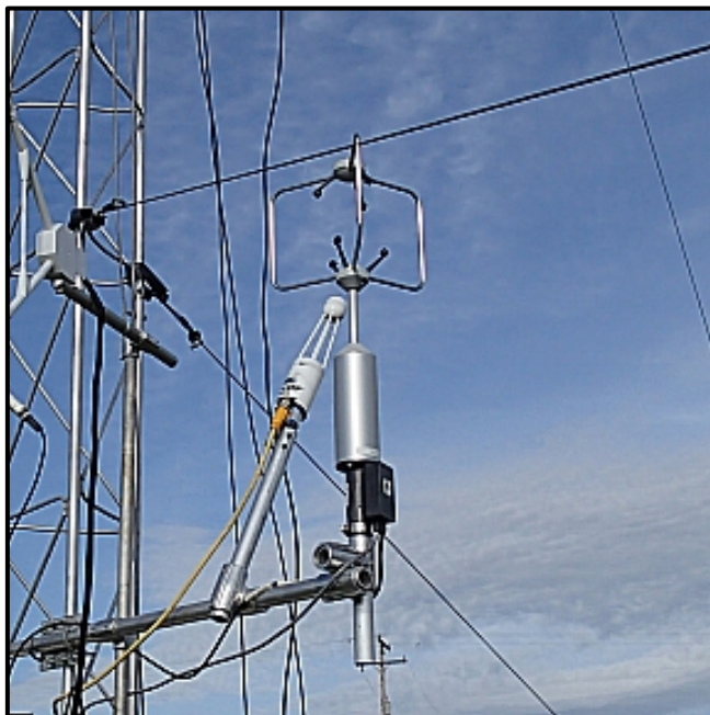
Figure 3-3 LI7500A with a Gill Anemometer
