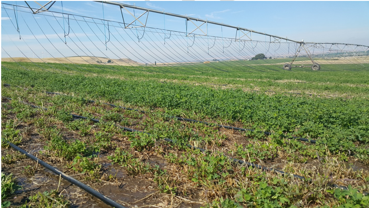
Figure 60. Mobile Drip Irrigation (MDI) in an alfalfa field.
