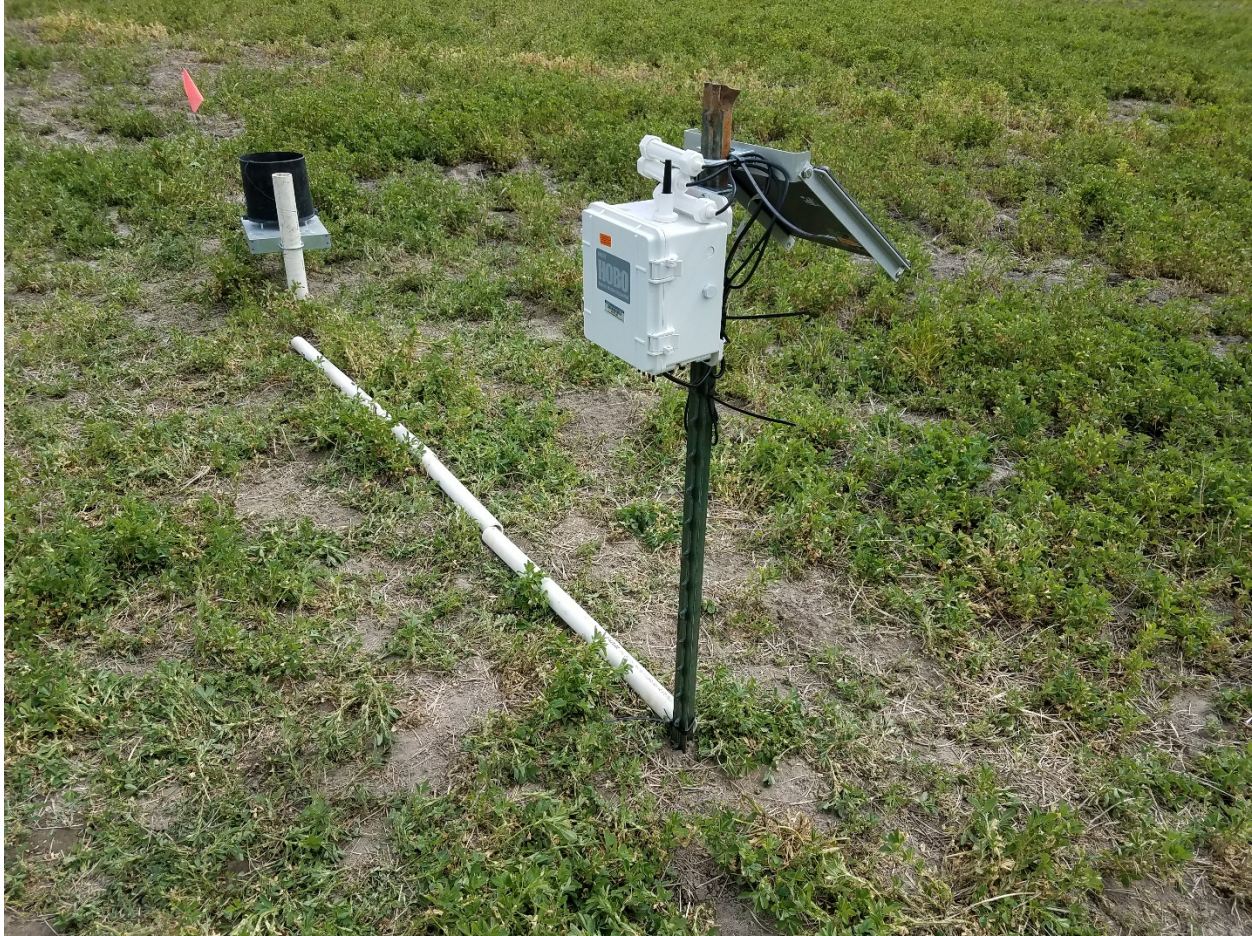
Figure 36. A soil moisture sensor installation in a field with telemetry and a rain gauge to measure applied water.
