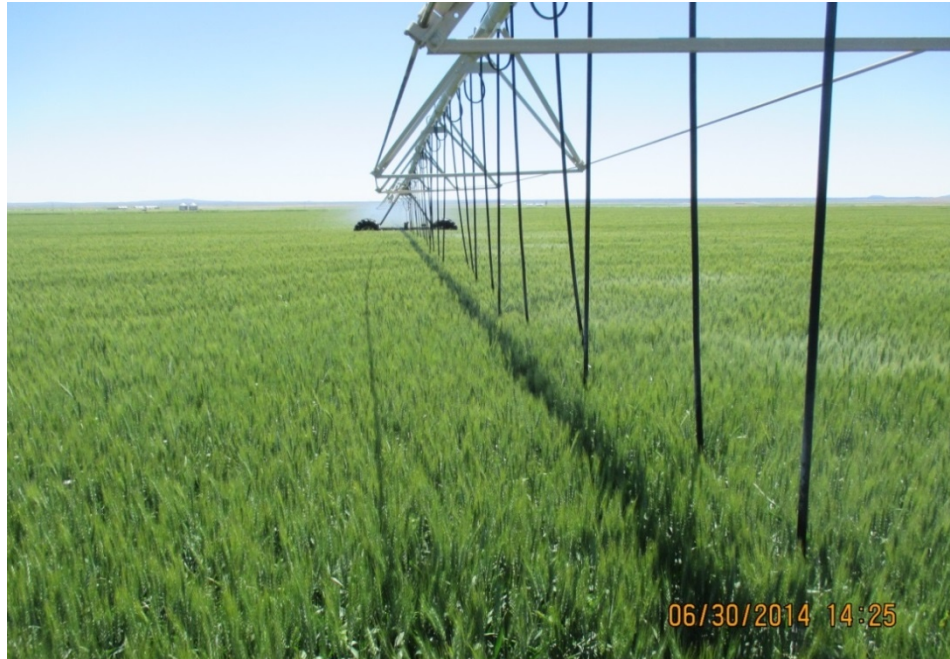
Figure 53. LESA operating in wheat with the sprinkler heads below the top of the canopy.
