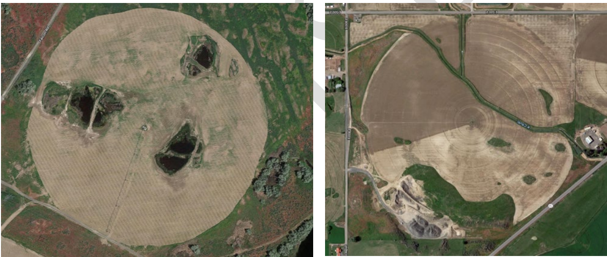
Figure 45. Using VRI on fields like these to avoid irrigating the non-cropped surfaces would certainly save water.
