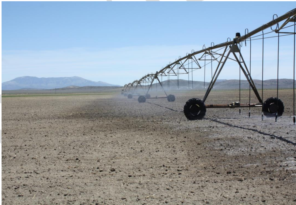
Figure 59. Due to its smaller wetted diameter, LESA allows less time for water to infiltrate into the soil. Therefore LEPA or LESA may not be suitable to tight soils or steep slopes where infiltration and runoff can be an issue.
