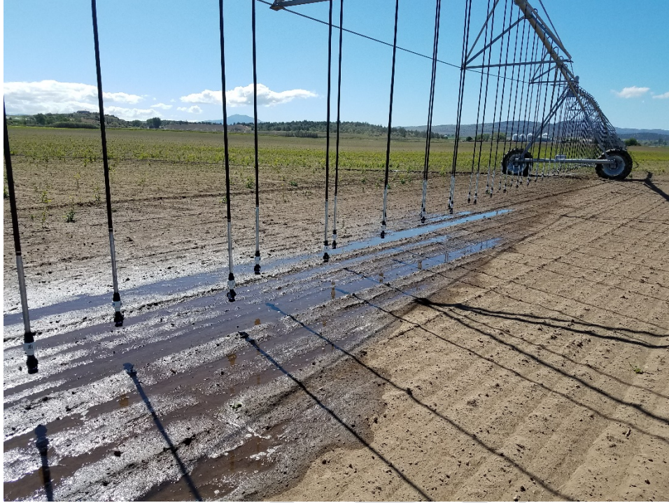
Figure 58. The application rate of LESA and LEPA is much higher than that for MESA. This can lead to increased runoff especially on bare soils, steep slopes, and heavier soils.
