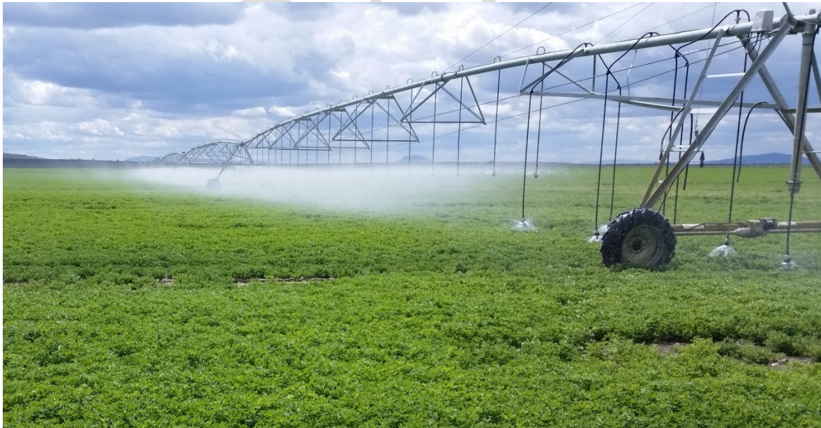
Figure 49. Water losses in the MESA section to the wind are visible, where no water losses can be seen in the LESA section of this pivot.
