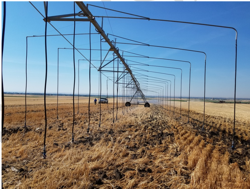
Figure 54. LESA system using boombacks to spread the water out and increase infiltration on a wheat field near Milton Freewater, Oregon.
