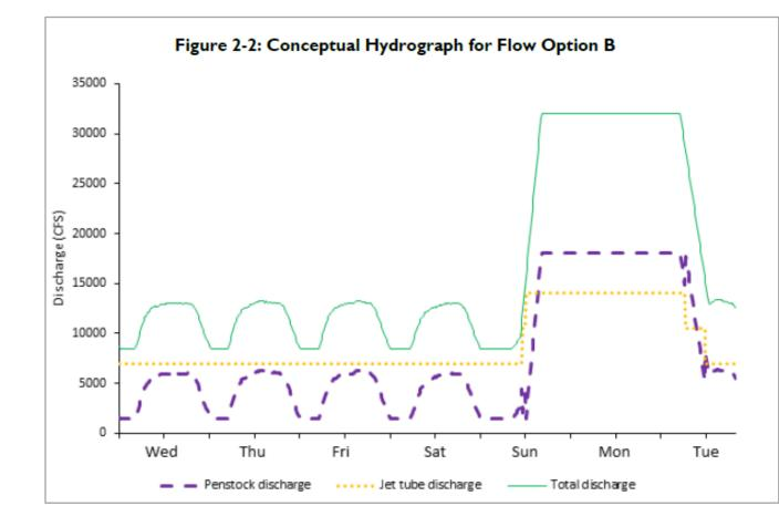
Similar to Flow Option A but would include **up to three 36-hour flow spikes** between late-May and mid-July **if sufficient water is available**
