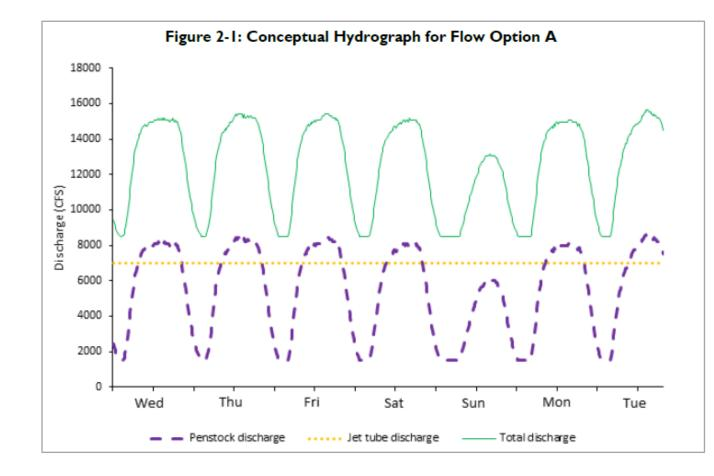
Water is released from both penstocks and bypass tubes to maintain a daily average water temperature below 16°C from below the dam to the confluence with the Little Colorado River (LCR)
