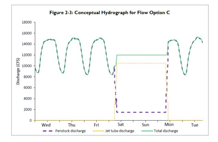
Once a week for at least 48 hours, switch to the minimum amount of byass needed to create a cold shock (13°C) all the way to the LCR
