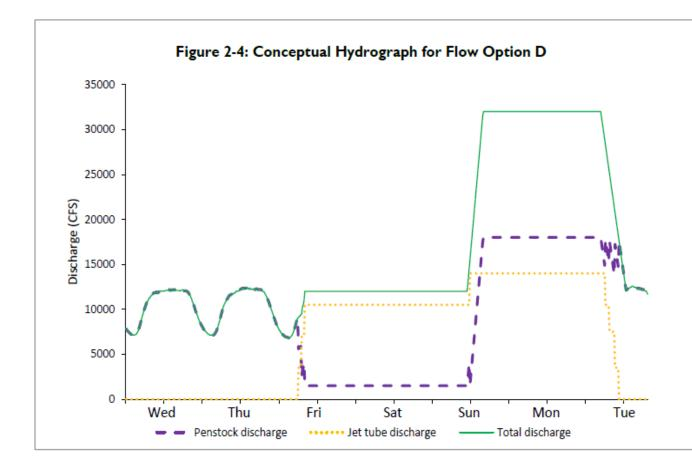
Similar to Flow Option C but would include **up to three 36-hour flow spikes** between late-May and mid-July **if sufficient water is available**.
