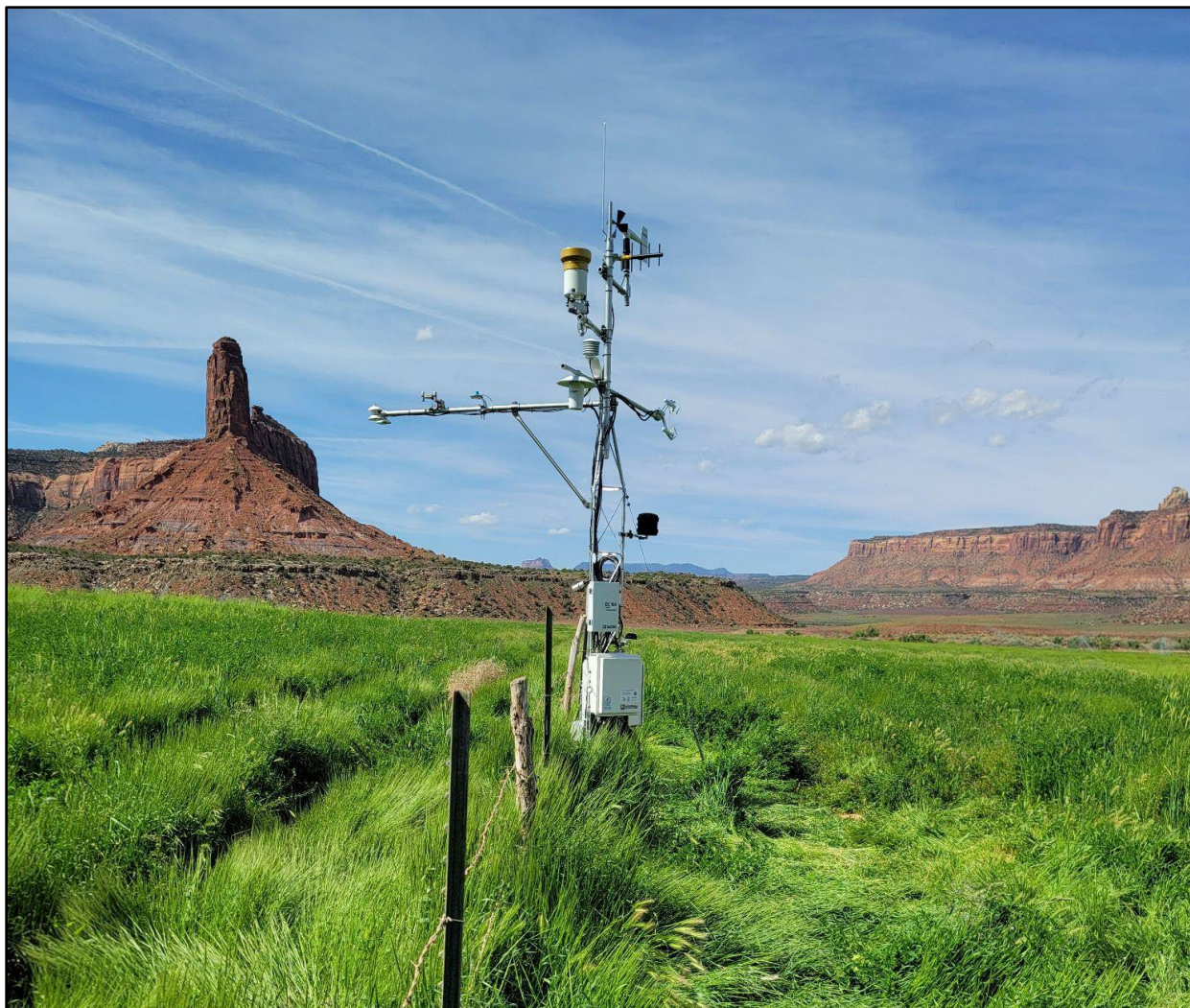
Figure 1. EC Tower installed at Dugout Ranch, part of the Canyonlands Research Center
