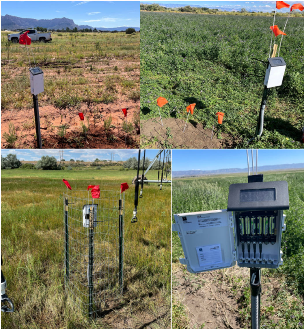
Figure 2. Soil sensors installed and soil data loggers in fields during the 2023 growing season.
