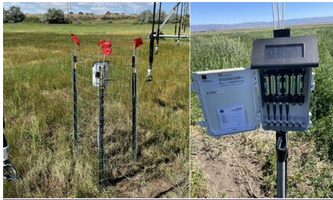
Figure 6. Soil sensors and data logger installed in fields during the 2023 and 2024 growing seasons
